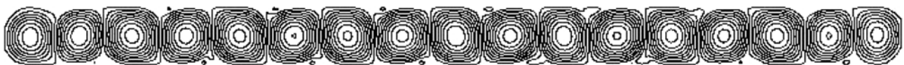
Fig. 2. Coexistence of large cells and a smaller-scale flow at R \approx 10R_c and P = 1 in the case of a rigid upper boundary; a = 20 , n = 20 . Streamlines (contours of the stream function) are shown.
